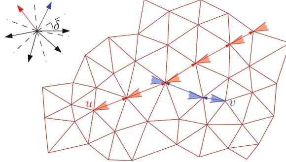
**Fig. 6.** Two vertices  $u$  and  $v$  that need to be extreme in two directions that differ by at most  $2\delta$  (indicated by red and blue) define a unique potential convex chain since there can be at most one edge in each sector
