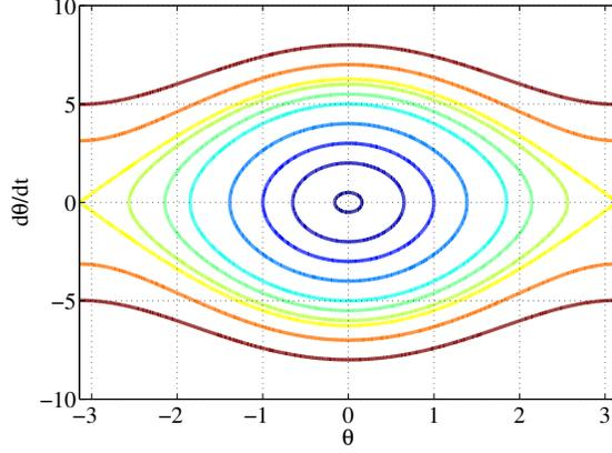
Figure 5: Phase portrait for the simple pendulum ( $l = 1$  and  $g = 9.8$  was used for this figure)
