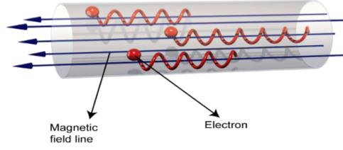
Figure 6: Helical trajectories of electrons immersed in a uniform magnetic field
