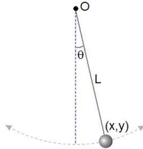
Figure 4: Schematic of the simple pendulum
