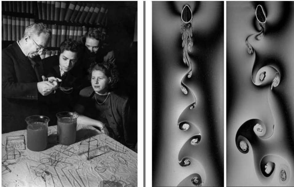
FIGURE 1.1. Richard Courant (left) using a suspended soap film to illustrate minimal surfaces, circa 1946. Reproduced with permission of the Courant Institute, New York University. Right: In a flowing soap film, the wakes swept below a flexible loop embedded within the film [21]. The coupled fluid-structure system shows bistability, with a stationary state and an oscillatory state. Reproduced with permission of the authors.
