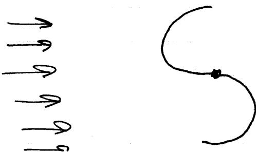
It should spin<sup>in</sup> a flow, thus forming a 2D turbine. You could easily apply a counter-torque, as if the turbine is turning a generator, and adjust the counter-torque to extract maximum power.
