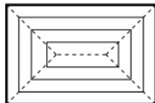
**Arrival time:** The function  $u(x) = \text{time of arrival to } x$  solves  $|\nabla u| = 1$  in  $\Omega$  with  $u = 0$  at  $\partial\Omega$
