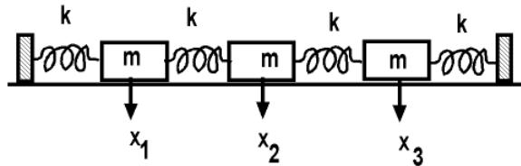
(a) We need to write down the system of three equations for  $x_1, x_2, x_3$ , the three displacements from equilibrium. The first of these is
